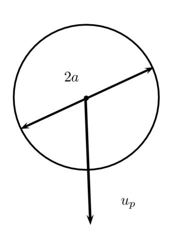
We calculate the drag force F exerted by an incompressible Newtonian fluid on a spherical particles with diameter 2r and density  $\varrho_p$ .
