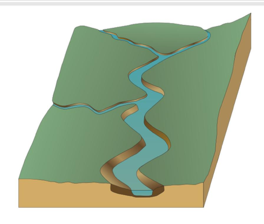
We are concerned with a water stream, whose variables are:  $\bar{u}$  [m/s], h [m], g [m/s<sup>2</sup>], and  $\theta$  [–]. The gravitational acceleration g and  $\theta$  are put together so that there are only n=3 variables. There are r=2fundamental units: m and s. Therefore, there is n-r=1 dimensionless group. This is the Froude number  $Fr = \bar{u}/\sqrt{gh\sin\theta}$ . The physics of water streams would entirely be embodied in the relation
