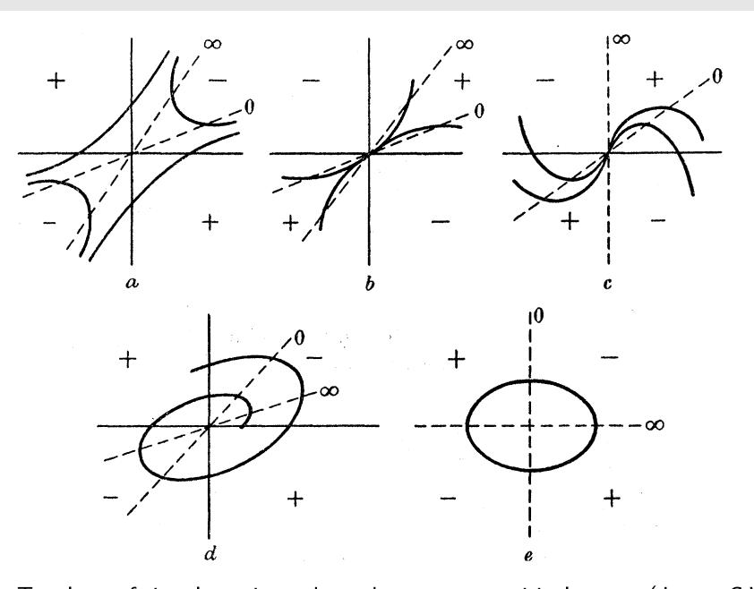
Typology of singular points where there are two critical curves (Jones, C.W., On reducible non-linear differential equations occurring in mechanics,, Proceedings of the Royal Society of London A, 217, 327-343, 1953.)
